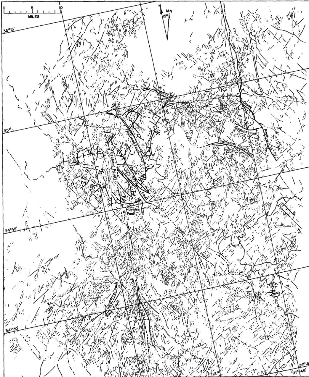
Figure 4a. Fault and lineament map of north-central Arizona. Faults compiled from published information. Lineaments are from monoscopic and stereoscopic analysis of EIOT4-I7375.
