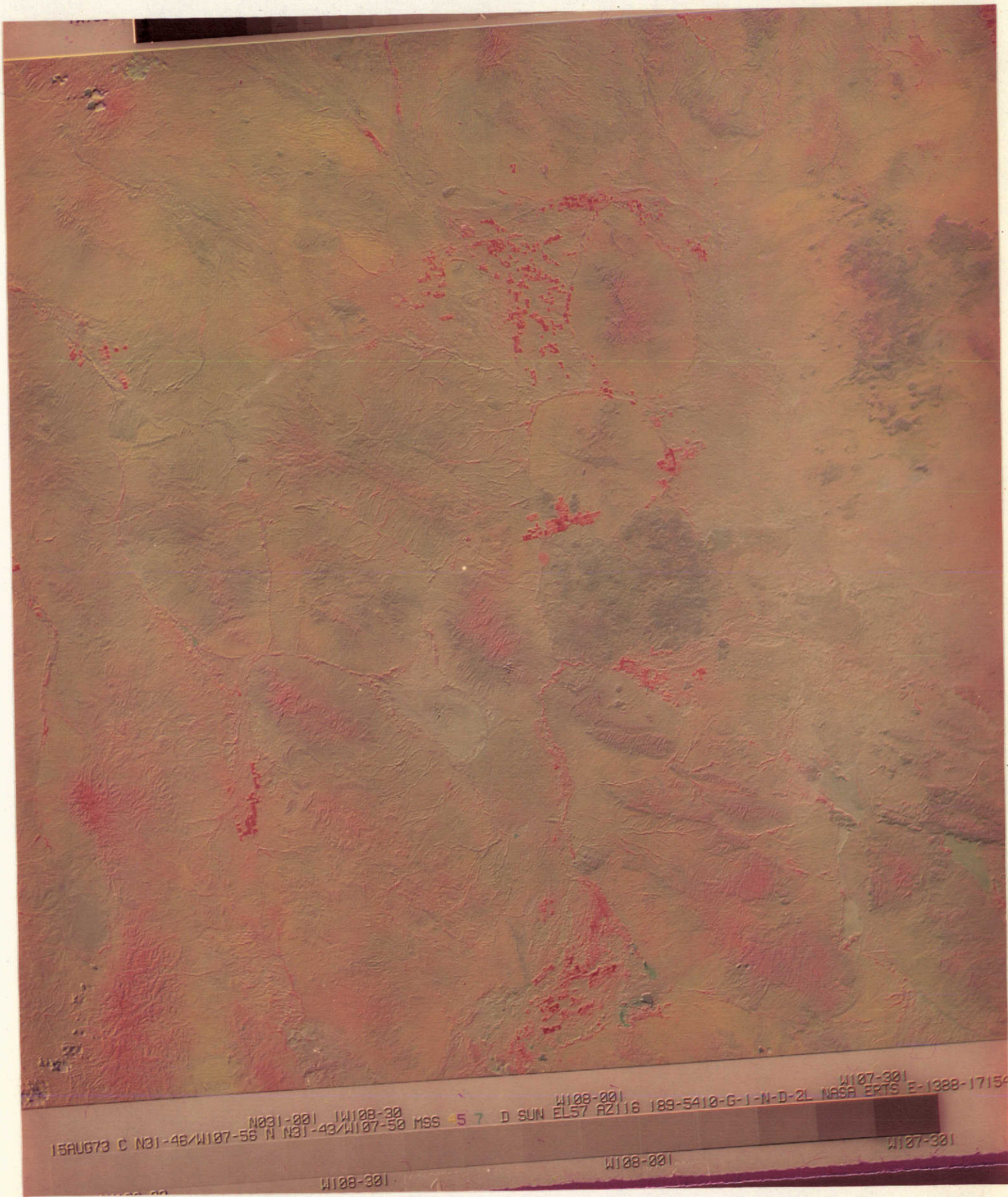
Figure 11. An isoluminous direct projection utilizing gamma "one" release positives of 15 August 1973 imagery. Band 4 is projected as blue, band 5 as green, and band 7 as red. The isoluminous process removes brightness differences from the image, leaving only color differences.
