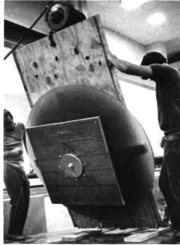
B. Transporting primary to polishing machine after the curve on the back had been generated.
