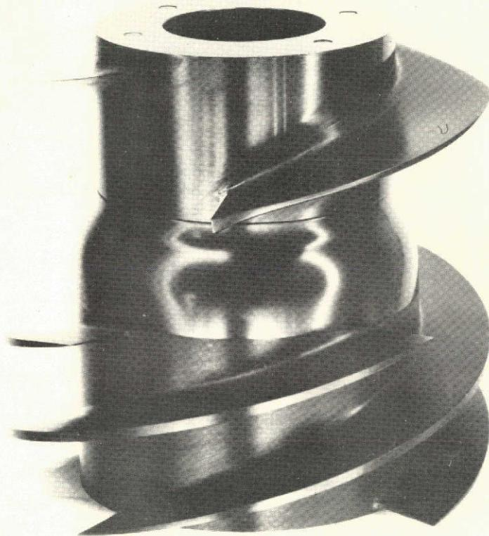
FIGURE 15 - TWO STAGE INDUCER ASSEMBLY
