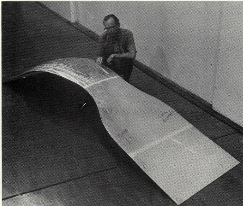
Figure 2-14. Gore Blank B Showing Weld
