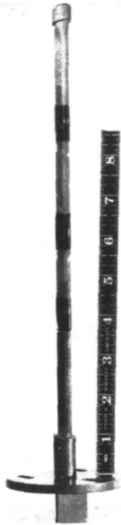
Inlet hot-film probe
