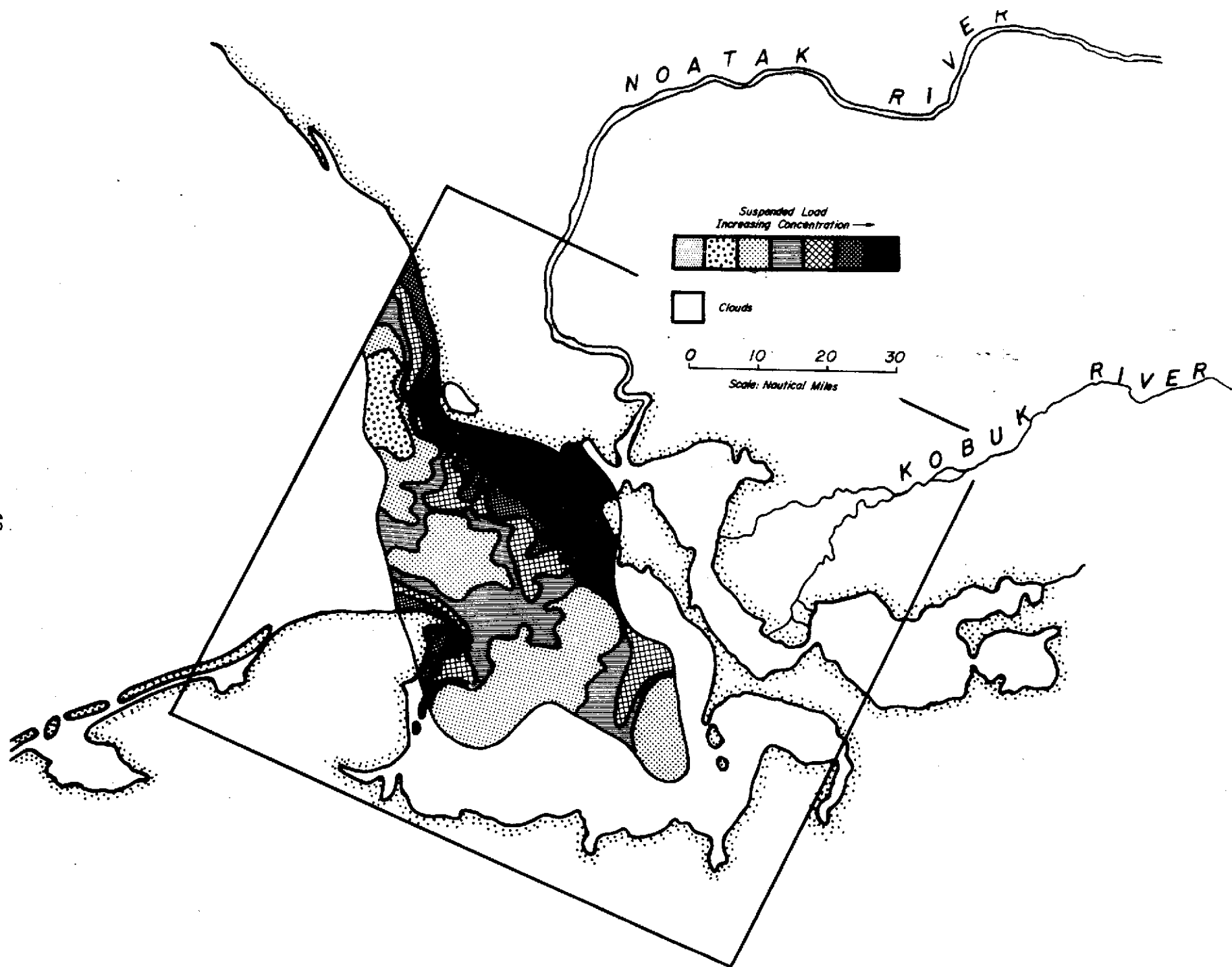
FIGURE 6. Relative suspended load distribution in the vicinity of Kotzebue Sound on 12 Aug 1973, based on color density slice of image I.D. 1385-21580-4. Refer to area 4 of Figure 1.
