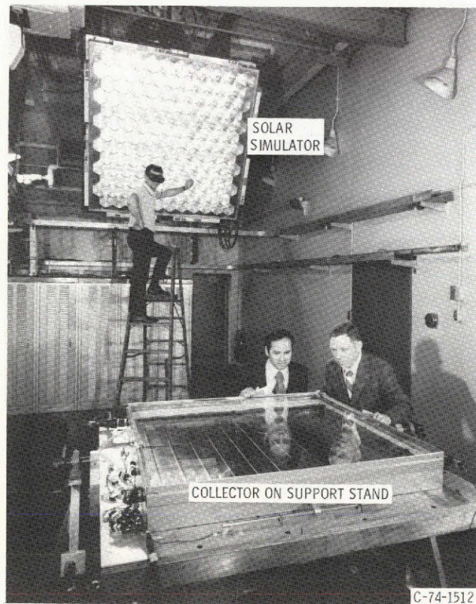
Figure 2. - Indoor facility used to experimentally determine solar collector performance.
