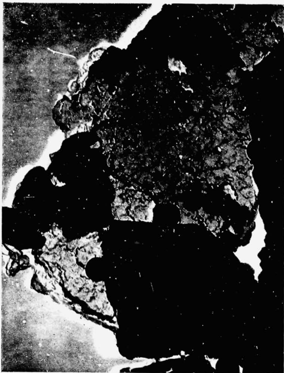
FIG. 7. Electron micrography of Iceland spar crystals ground for 50 hr (0.26 \mu\text{m} latex beads).
