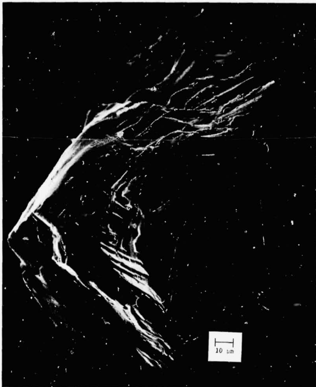
FIG. 4. Scanning electron micrograph of a prismatic crystal of a pyroxene mineral found in the Apollo 12 fines 12070 at 1000 magnification.
