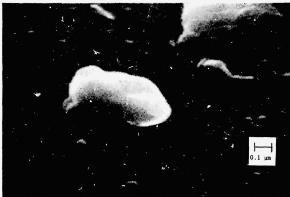
FIG. 3. Scanning electron micrograph of a small glassy area found on a particle from the Apollo 12 fines 12001 at 100,000 magnification.
