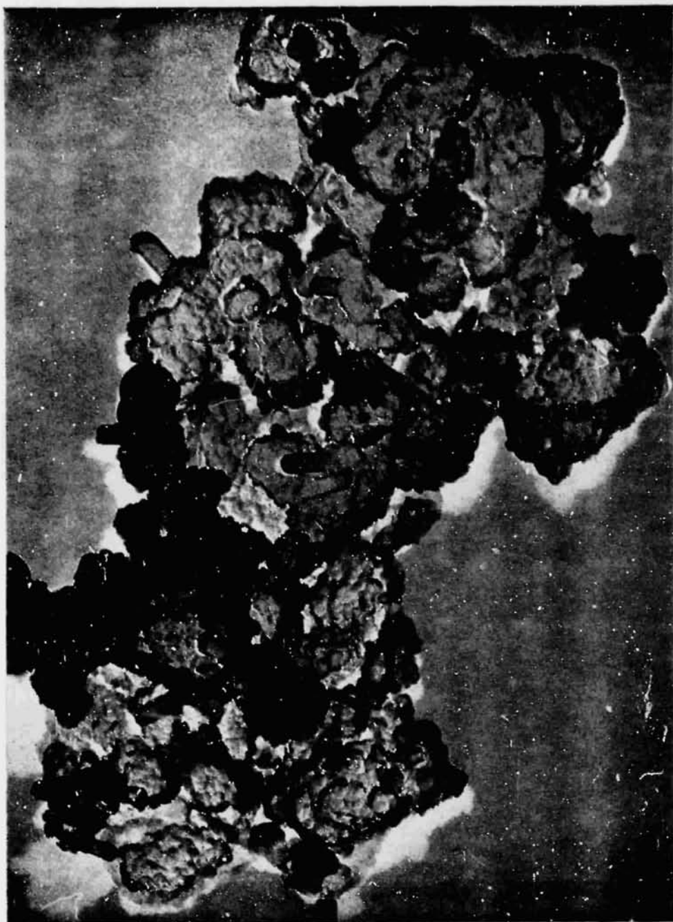
FIG. 15. Electron micrograph of 1000-hr calcite after treatment with water vapor, showing the whiskers of nail-head spar (0.26 \mu\text{m} latex heads).
