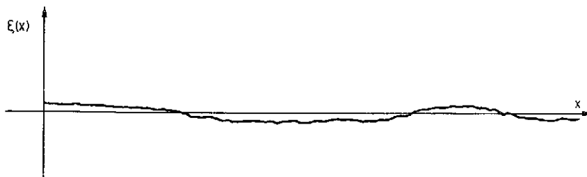
Figure 7. - Typical profile containing primarily medium-frequency components superimposed on a signal with low frequency.
