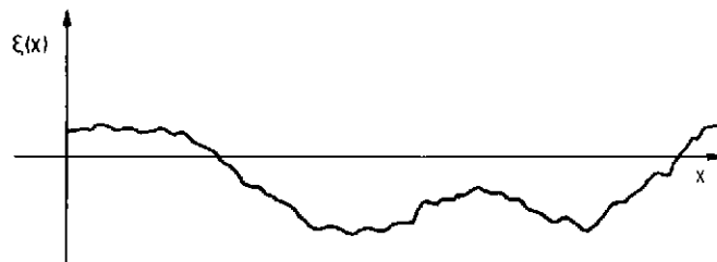
Figure 6. - Typical profile with high frequencies of small amplitude superimposed on a low-frequency signal.
