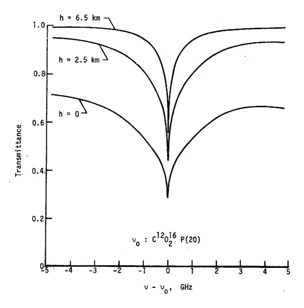
Figure 4.- Calculated frequency variation for tunable  $\mathrm{C}^{12}0_2^{16}$  laser for vertical transmittance from various altitudes.
