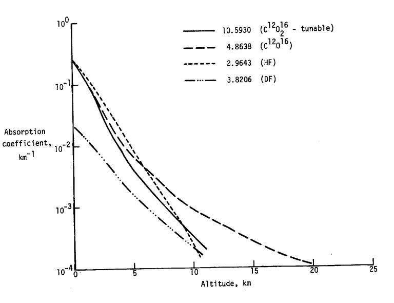
Figure 3.- Comparison of altitude dependence of absorption coefficients for tunable  ${\rm C}^{12}{\rm O}_2^{16}$  laser with CO, HF, and DF lasers.
