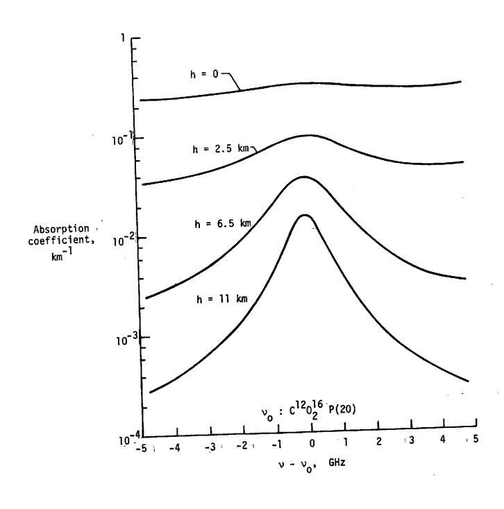
Figure 1.- Calculated frequency variation of absorption coefficient with altitude.
