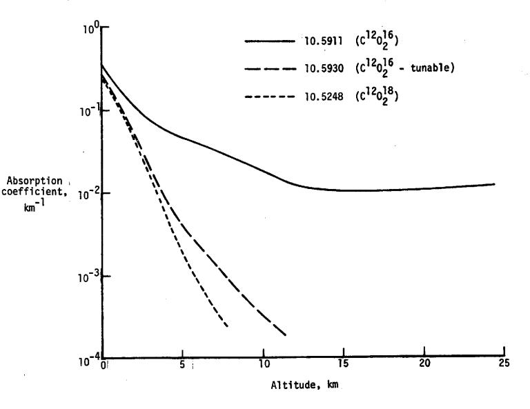
Figure 2.- Comparison of altitude dependence of absorption coefficients for CO<sub>2</sub> laser types.
