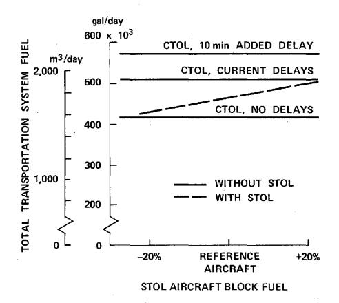
Figure 9.-Sensitivity of system fuel to STOL block fuel and CTOL air delay.
