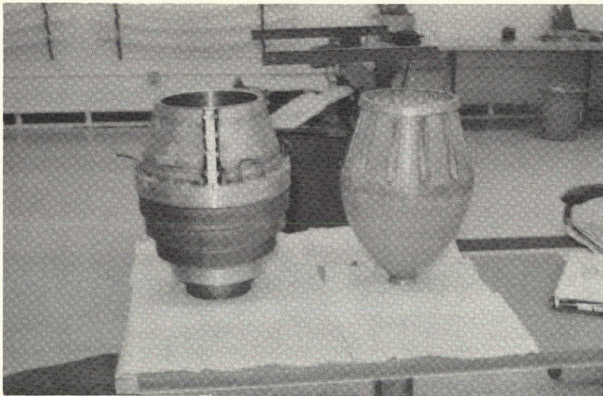
Figure 3.2-3. Ogive Radome and Fabrication Mold
