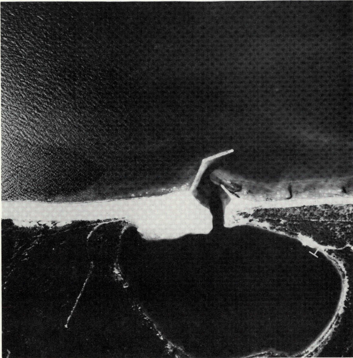
FIGURE 3. LITTLE LAKE HARBOR, 7 MAY 1974. Since its original construction on the south shore of Lake Superior, shoaling problems have been experienced at Little Lake Harbor. This photograph, providing the first good vertical view of the harbor since 1964, clearly shows the transport of material from the east and the continuous nature of harbor mouth shoaling effects from the sandbar outside the harbor. The resulting sediment transport patterns produce rapid shoaling in the mouth of the harbor, making it difficult to maintain the desired 4m depth. This photograph is expected to be very useful for a design-deficiency study scheduled to begin in FY 75. (Original in color.)
