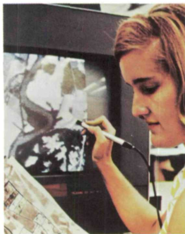
Analyst uses a light pen to outline a training field on a cathode-ray tube (CRT) display. The computer will use data gathered by field observers to compare this field to others on the data tape.
