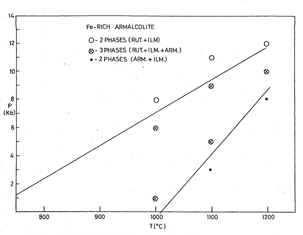
Figure 3: Comparison of P-T stability of synthetic armalcolite ((Fe.5 Mg.5)Ti205) with whole rock liquidus curve determined by Akimoto et.al. (1970) for an armalcolite-containing Apollo 11 rock.
