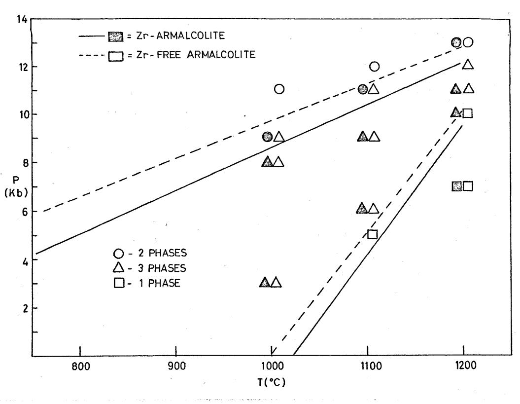
Figure 2: P-T stability of armalcolite prepared in equilibrium with metallic iron.
