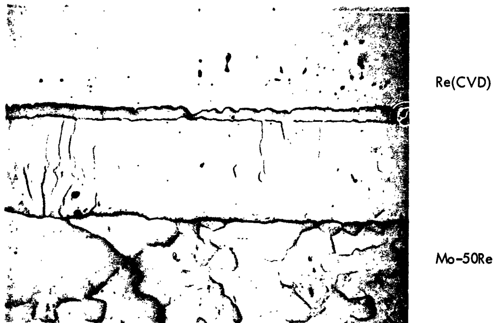
Figure 68. The Molybdenum-50Rhenium to CVD Rhenium Interdiffusion Zone After Ageing at 1800°C for 1000 hours (41A-5) at 200X
