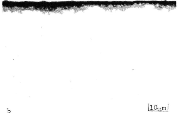
FIGURE 7. SCALE FORMED ON Ti-25Cr-8Al AFTER  $1.8 \times 10^5$  s (50 h)
