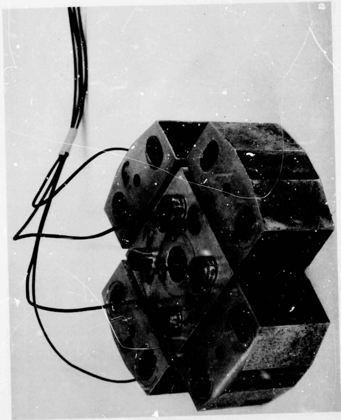
Fig. 7 Test Assembly of Four Elastomer Shear Specimens, Each 2.54 cm (1.0 in.) High
