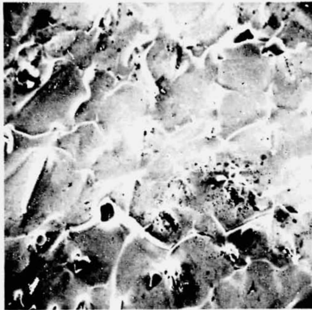
Figure 41. Scanning electron micrograph of the resolidified surface of Specimen SL-2.5 near the sting side (250X).
