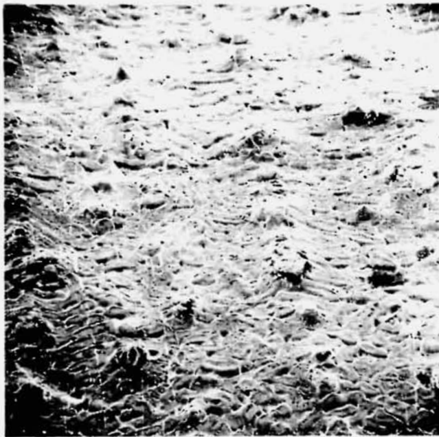
Figure 17. Scanning electron micrograph of the columnar dendrites on the surface of Specimen SL-1.8 (250X).
