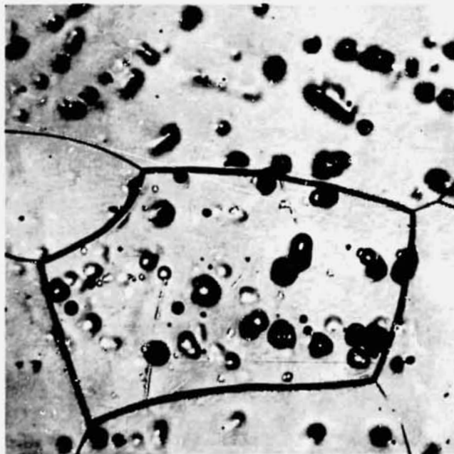
Figure 38. Optical micrograph of the microstructure near the sting on the cross section of Specimen SL-1.9 (100X).
