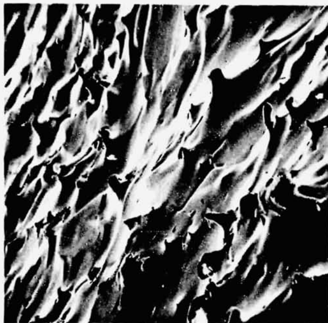
Figure 47. Scanning electron micrograph of the resolidified surface of Specimen SL-2.5 near the unmelted portion at the bottom of the specimen (250X).
