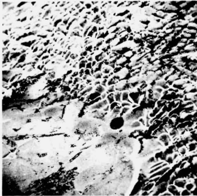
Figure 45. Scanning electron micrograph of an edge of the protrusion on Specimen SL-2.5 (250X).
