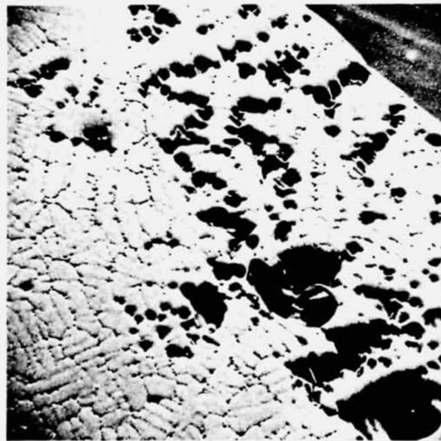
Figure 24. Scanning electron micrograph of the microstructure near the porous band in the cross section of Specimen SL-1.8 (100X).
