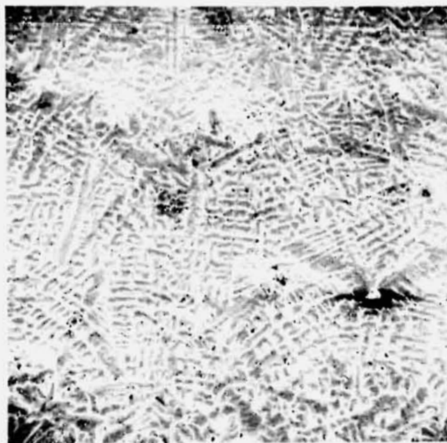
Figure 3. Scanning electron micrograph of the columnar dendrites on the surface of Specimen SL-1.3 (100X).
