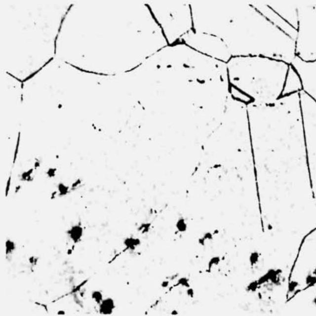
Figure 50. Optical micrograph of the etched cross section of Specimen SL-2.5 in the boundary between the resolidified and unmelted portion (100X).
