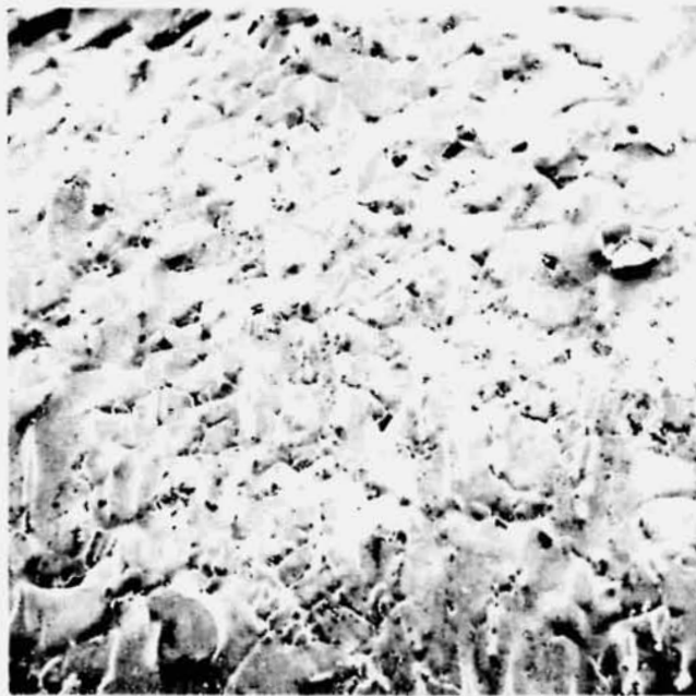
Figure 42. Scanning electron micrograph of the resolidified surface of Specimen SL-2.5 near the top (100X).
