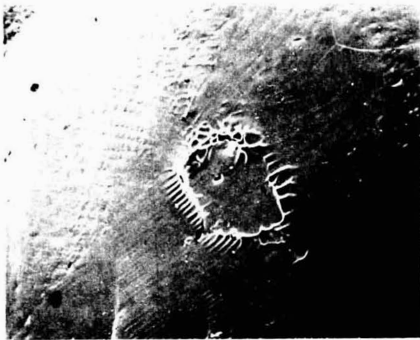
Fig. 3 Shallow Cavity on Surface Following Impact with Chamber Wall While Molten, Sample 1-15, Pure Nickel (150 \times )
