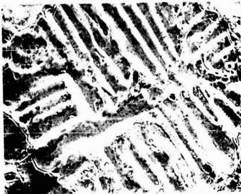
Fig. 13 Dendritic Grain in Cap Region, Showing Terraces, Sample 1-7, Ni-30Cu (750x)
