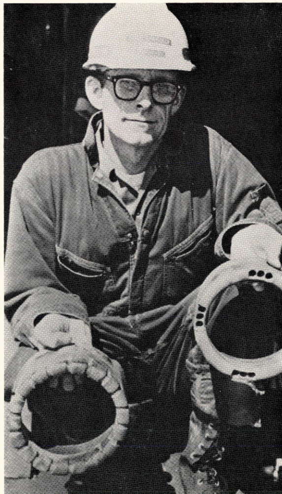
Two different type core bits used in taking core at Lyons, Kansas, Radioactive Waste Repository Site.
