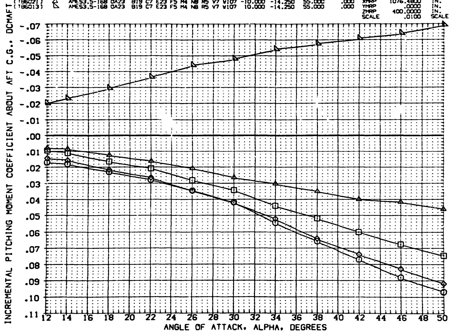
FIG. 7 ELEVON EFFECTS (B)MACH = 7.20 139B CONFIGURATION (0.010-SCALE).
