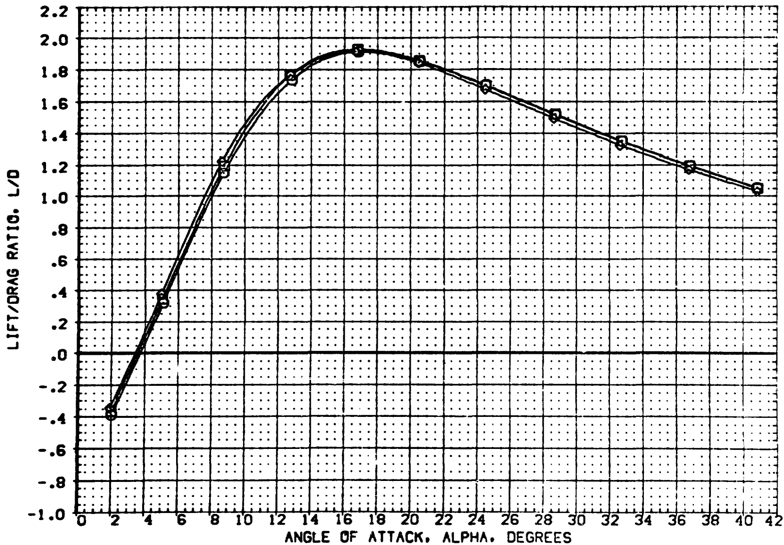
FIG. 5 BODY FLAP EFFECTS 147B CONFIGURATION (0.015-SCALE). (A)MACH = 5.26
