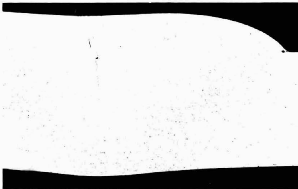
FIGURE A-10. PORES IN RAMP SECTION -H-1
