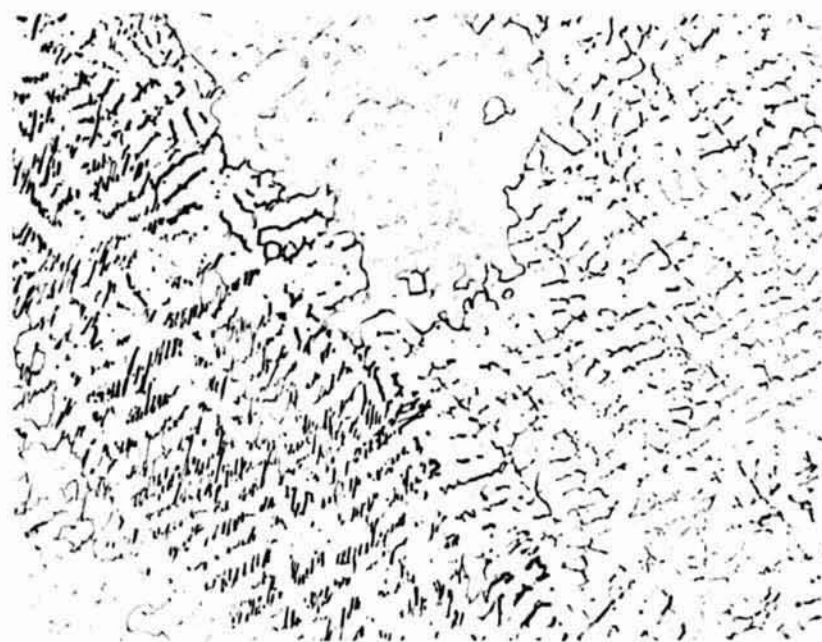
FIGURE B-28. INTERNAL MICROSTRUCTURES IN DWELL REGION - S/N 106 SKYLAB
