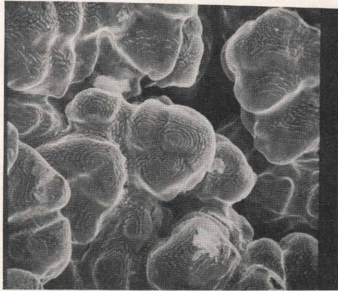
Figure 12. Micrograph Showing Decorated Growth Terraces of Sample 1-6 (1000X).
