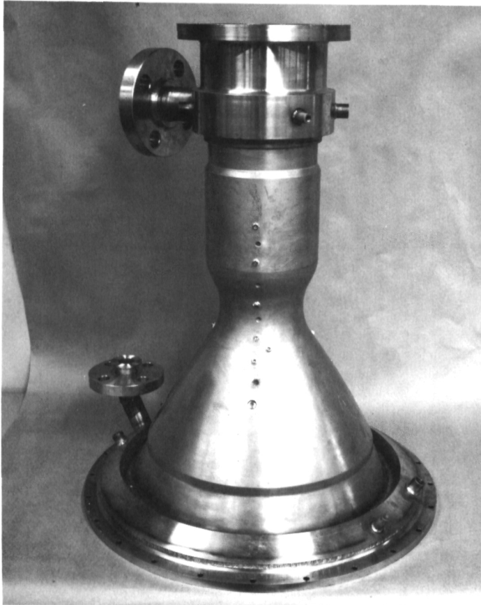
Figure 33. - Regeneratively cooled TD nickel-lined thrust chamber.
