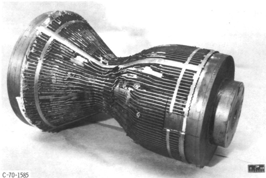
Figure 3. - Grown-rib structure torn loose during machining.
