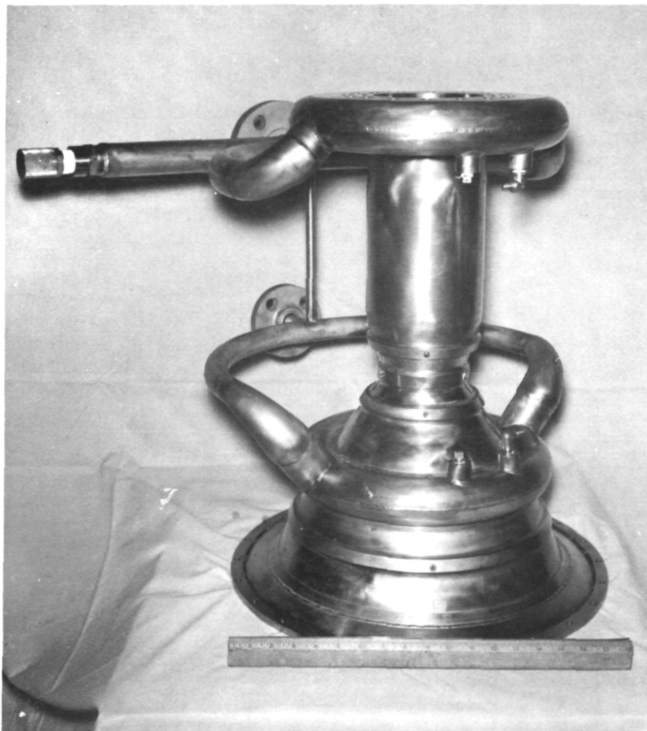
Figure 13. - Tungsten-lined thrust chamber with plumbing attached.
