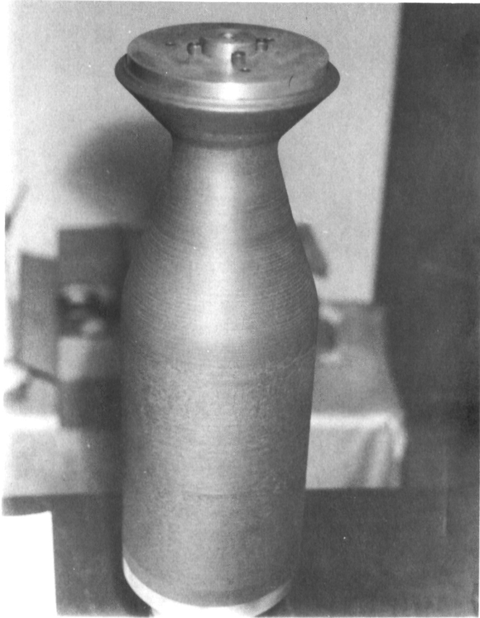
Figure 40. - Graphite sections after gluing and machining and before electroforming.
