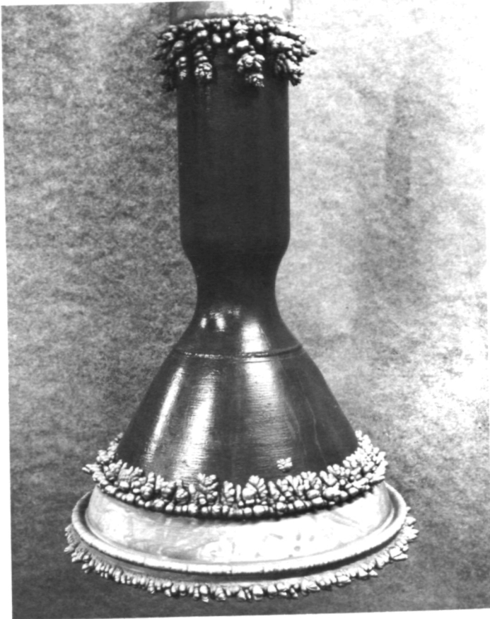
Figure 25. - Nodular growth during electroforming of flange ends.
