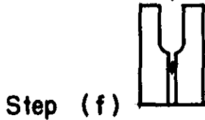
Fig. 7. Machining sequence for modified form of fracture specimen
