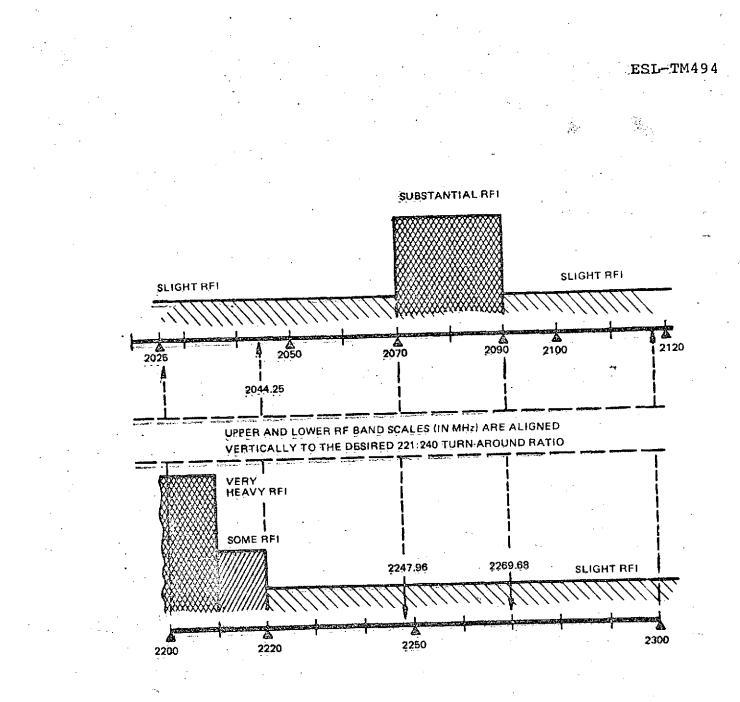
Figure 3-1. Relative RFI Densities Expected From Radars in the 2 to 2.3 GHz Band
