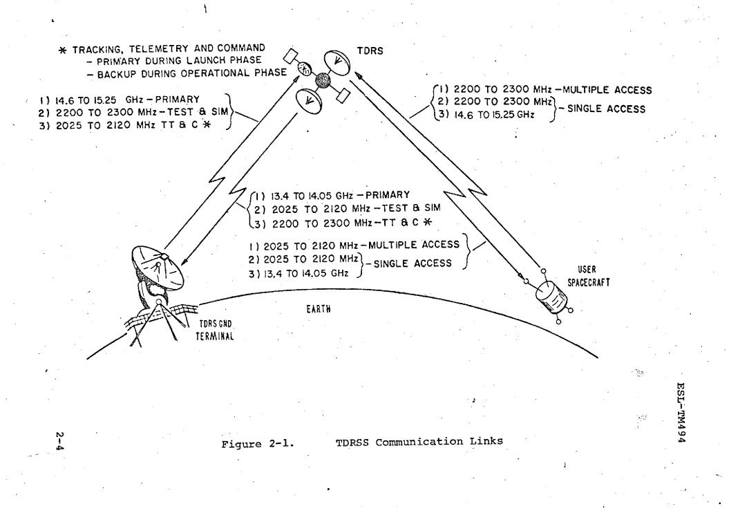
This study has focused on the spacecraft-borne receivers involved in the system, specifically: Table 2-2 Items RF Bands (GHz) То From Link D1, D2 and D3 14.6-14.87 TDRSS Ground Forward D5 15.15-15.25 A2 2.036 Al, A3 and A4 2.025-2.12 Users TDRS Forward C3 13.75-13.8 Bl, B3 and B4 2.2 - 2.3TDRS Users Return D4 14.896-15.121
