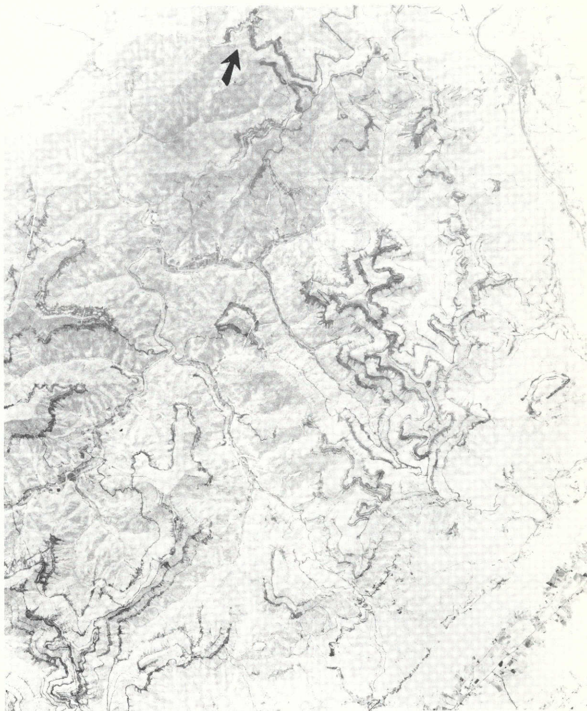
Figure 16. Strip mine signatures on a negative print of the Cumberland Plateau Test Site. RB-57 high altitude aircraft mission at 60,000'. Note the absence of strip mines indicated by the arrow as compared with the presence of strip mines for the same location on the ERTS frame in figure 17. 18 April, 1972. Mission 197 site 177, frame 26-0063.
