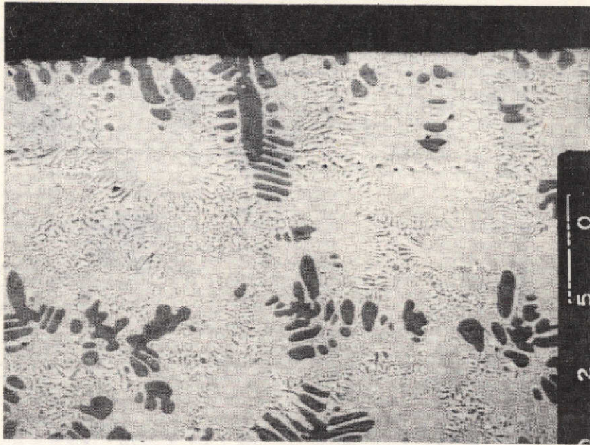
Figure 15. Scanning Electron Micrograph of SLS 3-28mm - 5° showing dendrites present in the ring-groove along with the complete absence of the primary silver phase shown in Figures 13 and 14. (250X)
