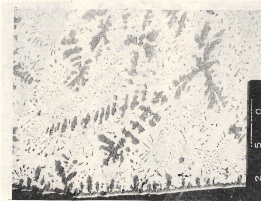
Figure 8. Scanning Electron Micrograph of SLN 4-5mm - 290° with a large dendrite. (250X)
