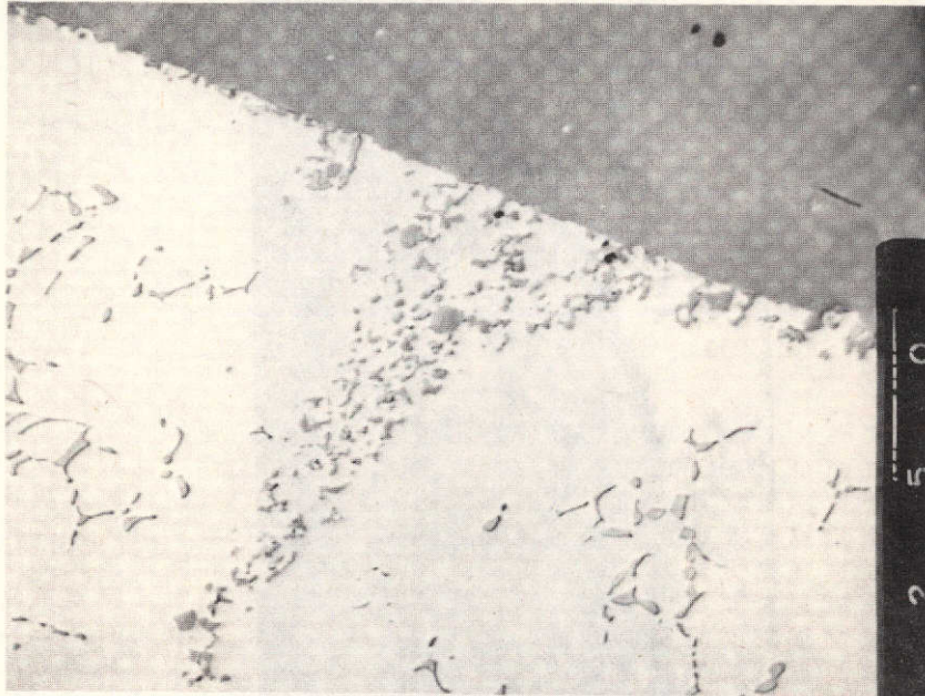
Figure 19. Scanning Electron Micrograph of SLS 3-12mm - 5° showing stainless particles in braze alloy. (500X)
