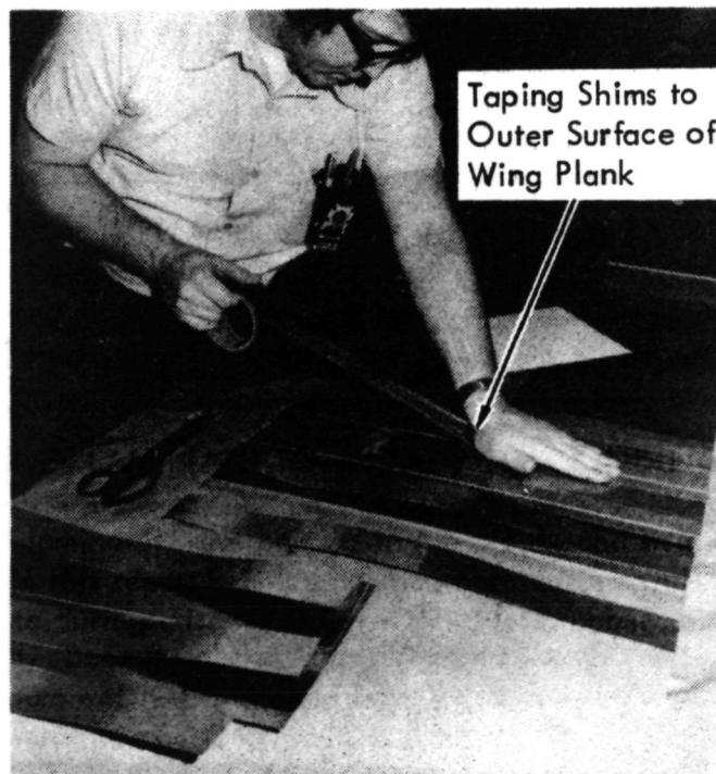
FIGURE 37. - SHIMMING OUTER SURFACE OF WING PLANK FOR BONDING
