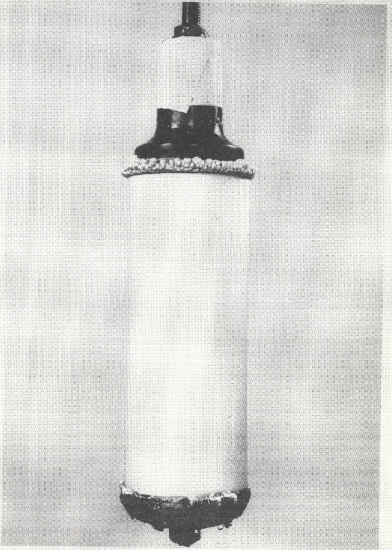
Figure 21. Fixtured Test Cylinder After Electroforming
