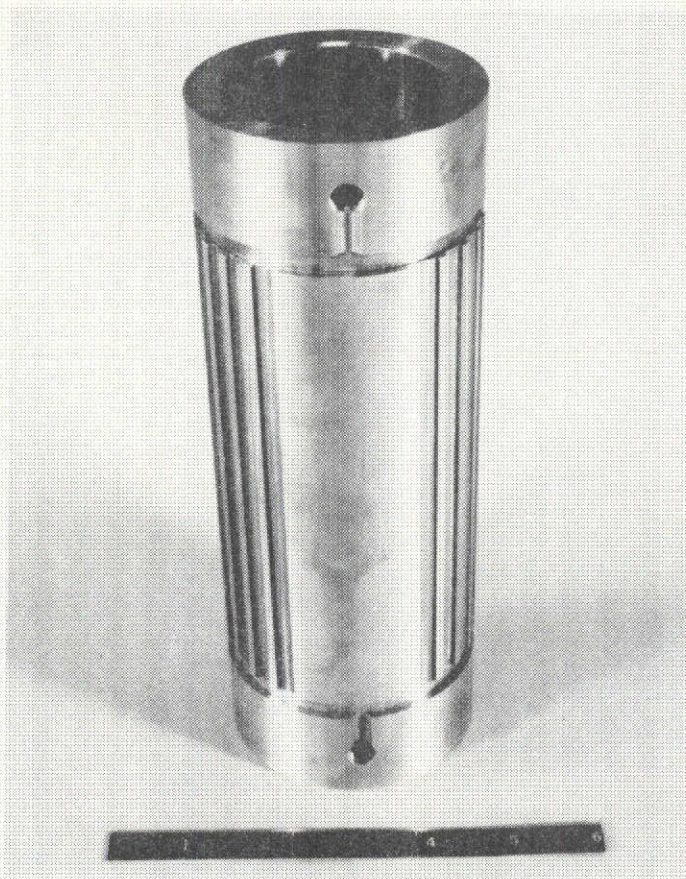
Figure 19. OFHC Copper Liner After Machining
