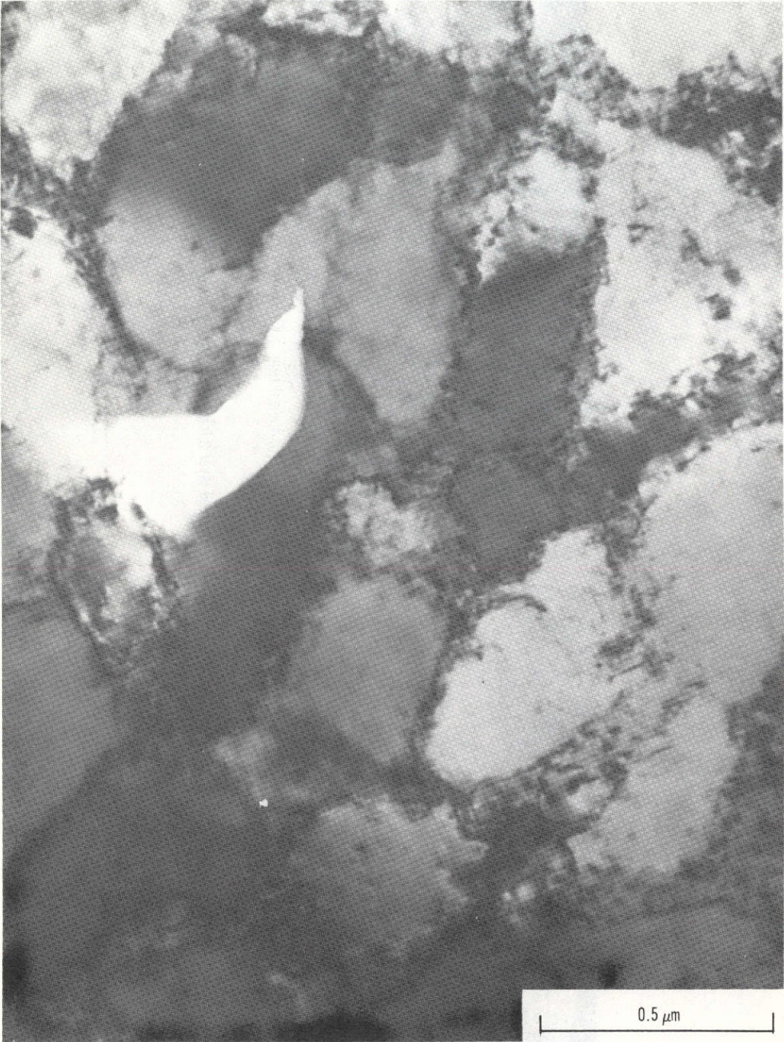
Figure 6. - Electron micrograph of copper subjected to sliding against 440C steel in liquid methane. Normal load, 1 kilogram; sliding speed, 6.2 meters per second; specimen made from metal adjacent to wear scar surface.
