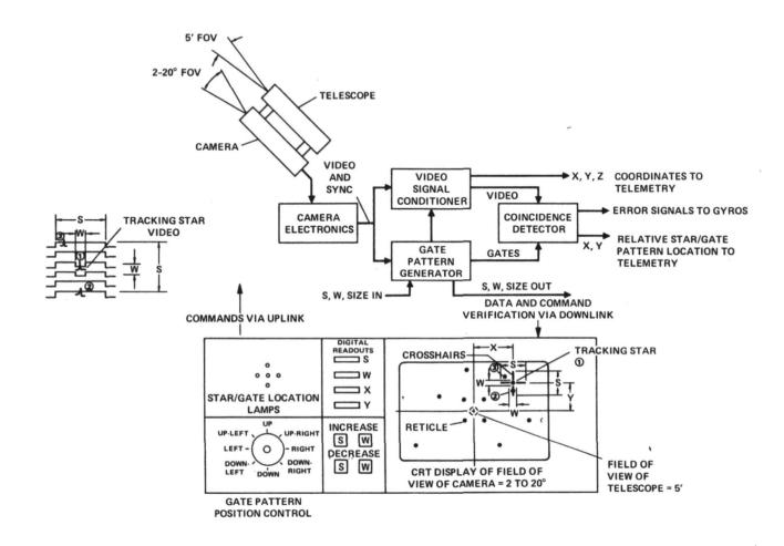
Figure 3. Offset tracking using gate generated crosshair
