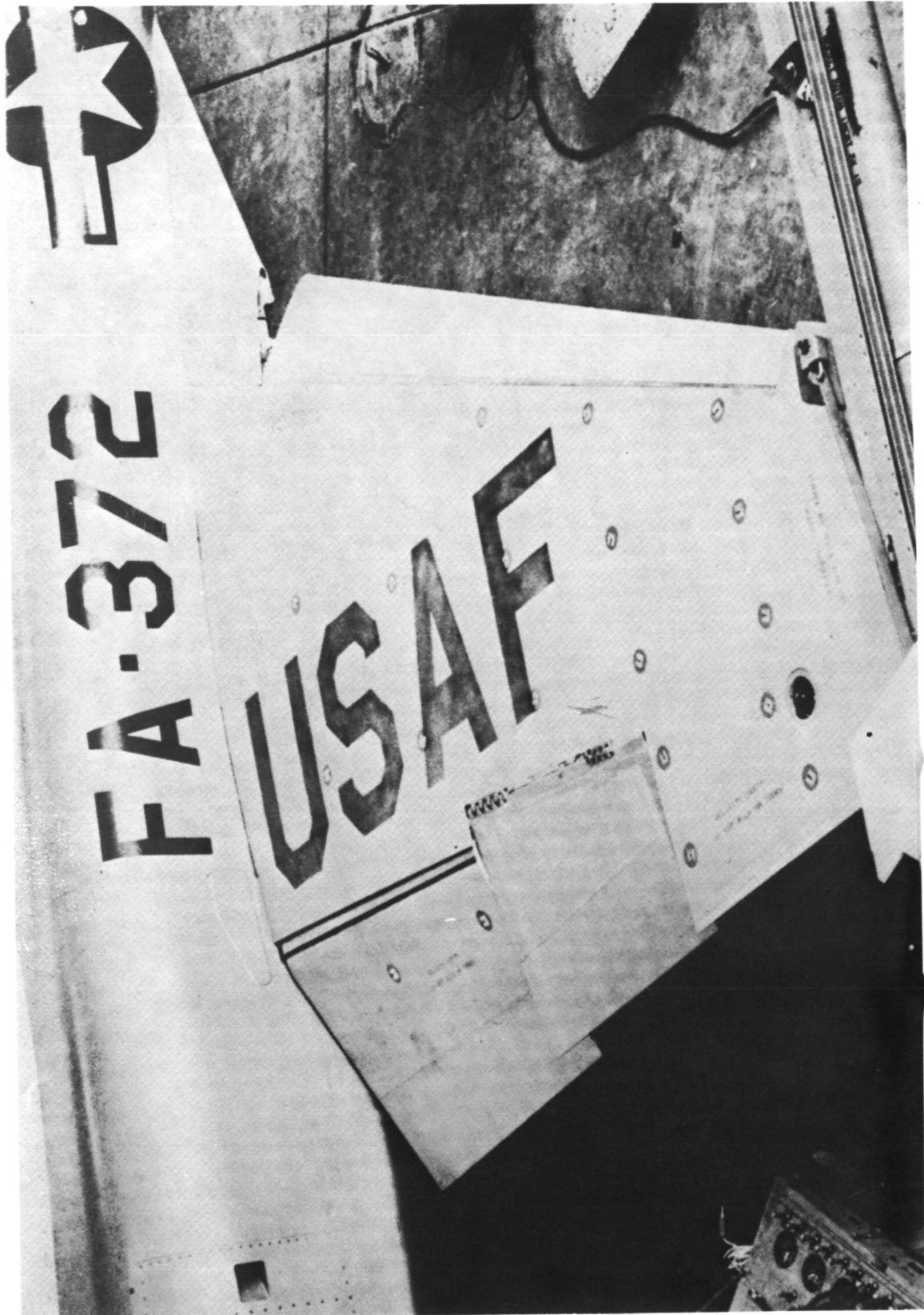
Figure 5. Right Wing of F-5A Aircraft After Installation of Dynamic Pressure Transducers
