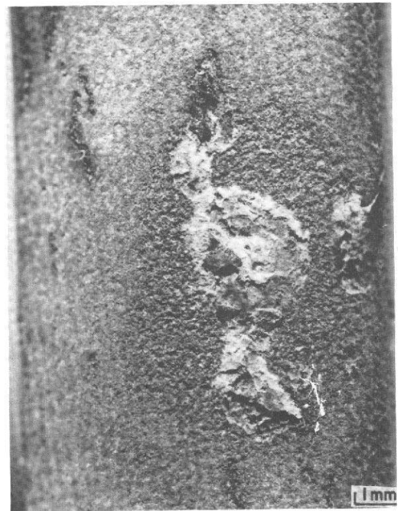
Figure 51 Surface Appearance of Thermal Fatigue Cracks in the Trailing Surface of NiCoCrAlY Coated \gamma/\gamma' - \delta Erosion Bar (R-7409) After Indicated Time in the Burner Rig 1366°K (2000°F) Cyclic Oxidation Test. Localized Oxidation Failures of the Coating Were Initiated at the Thermal Fatigue Cracks.
