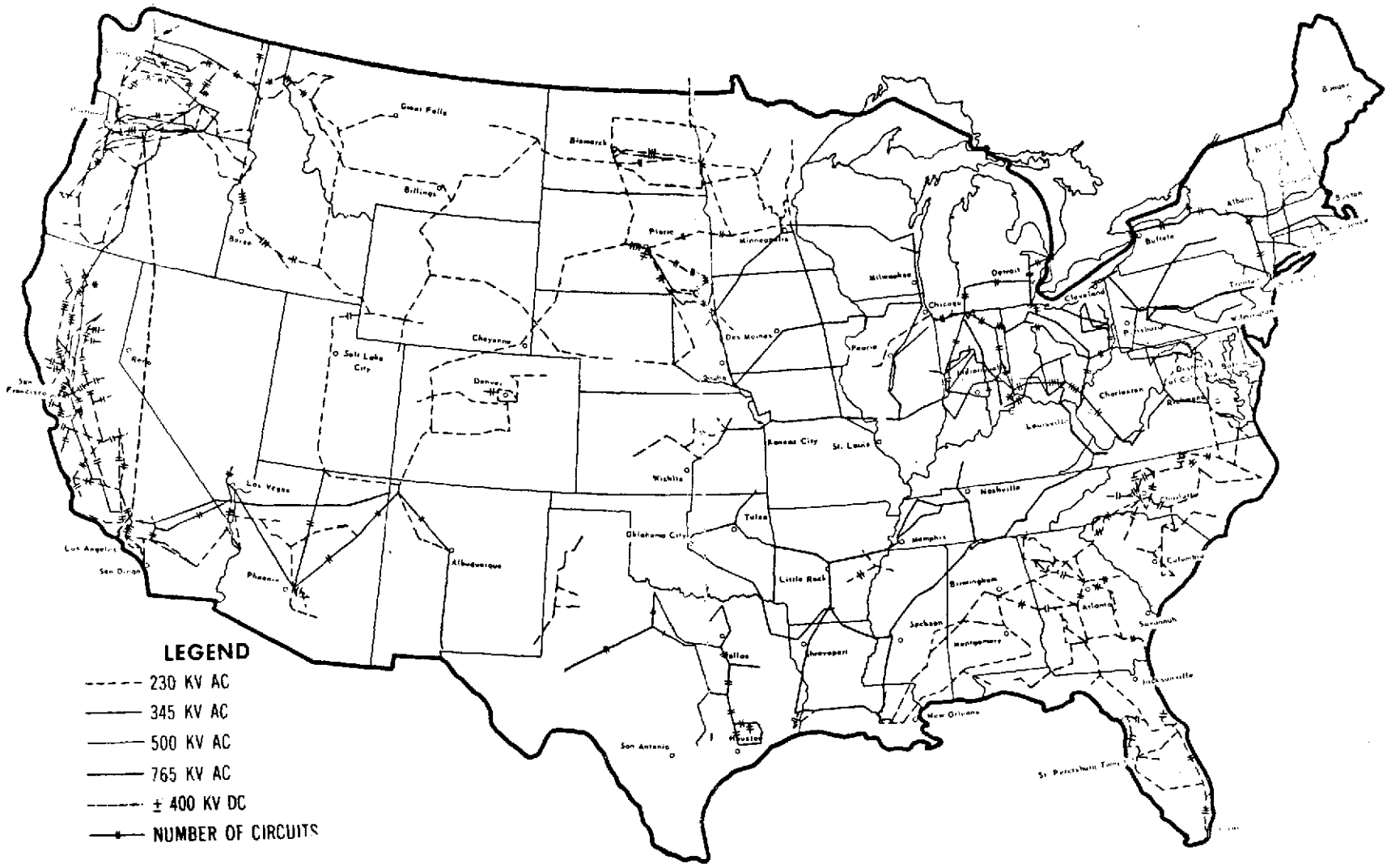
FIGURE D-5 1970 ELECTRIC TRANSMISSION SYSTEM [FPC-70]
