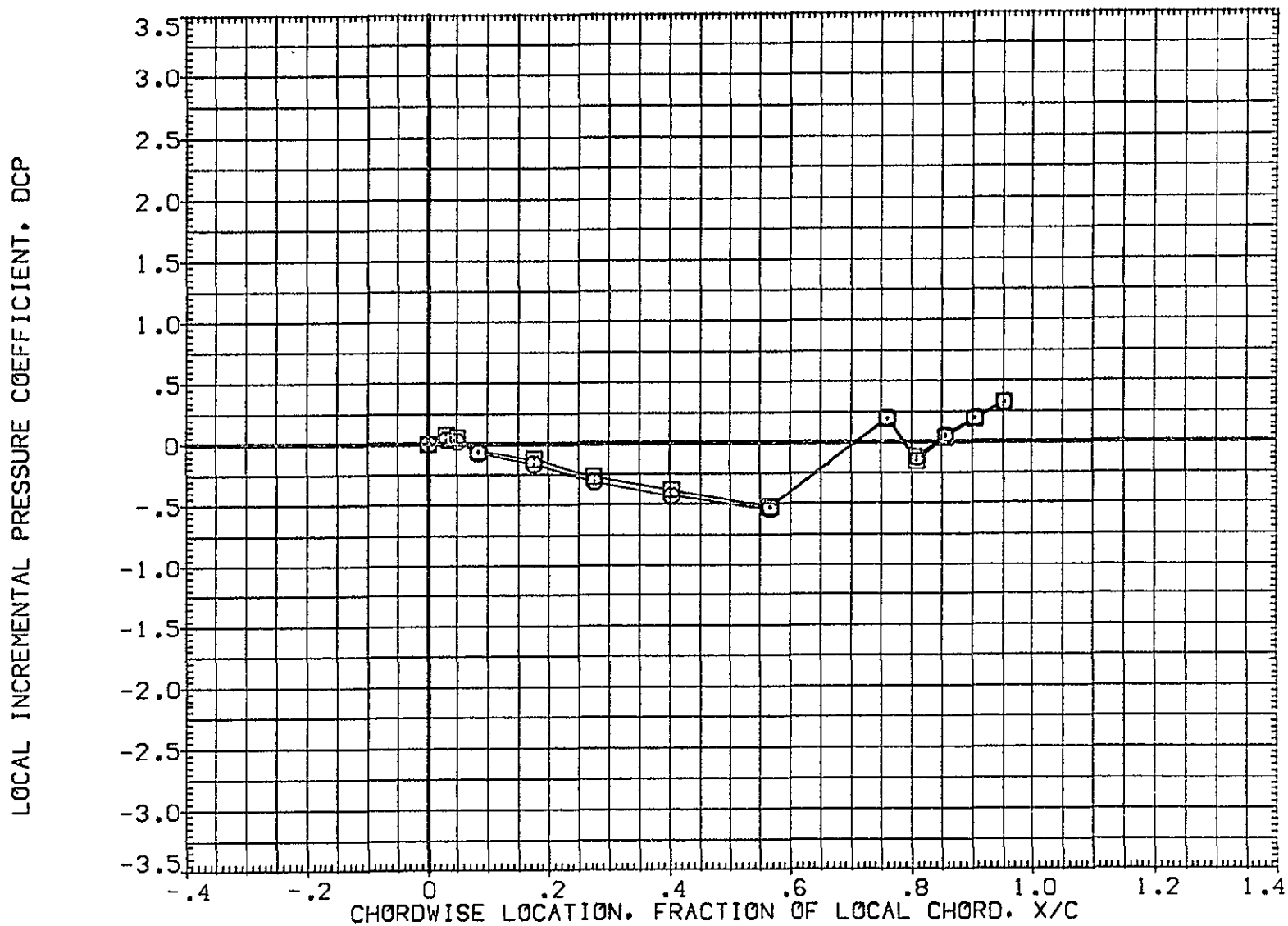
FIG 30 EFFECT OF FORWARD ATTACH POINT WEDGE, 8 DEGREE ELEVON DEFLECTION MACH = 1.240 ALPHA = .000 2Y/B = .436 PAGE 1321
