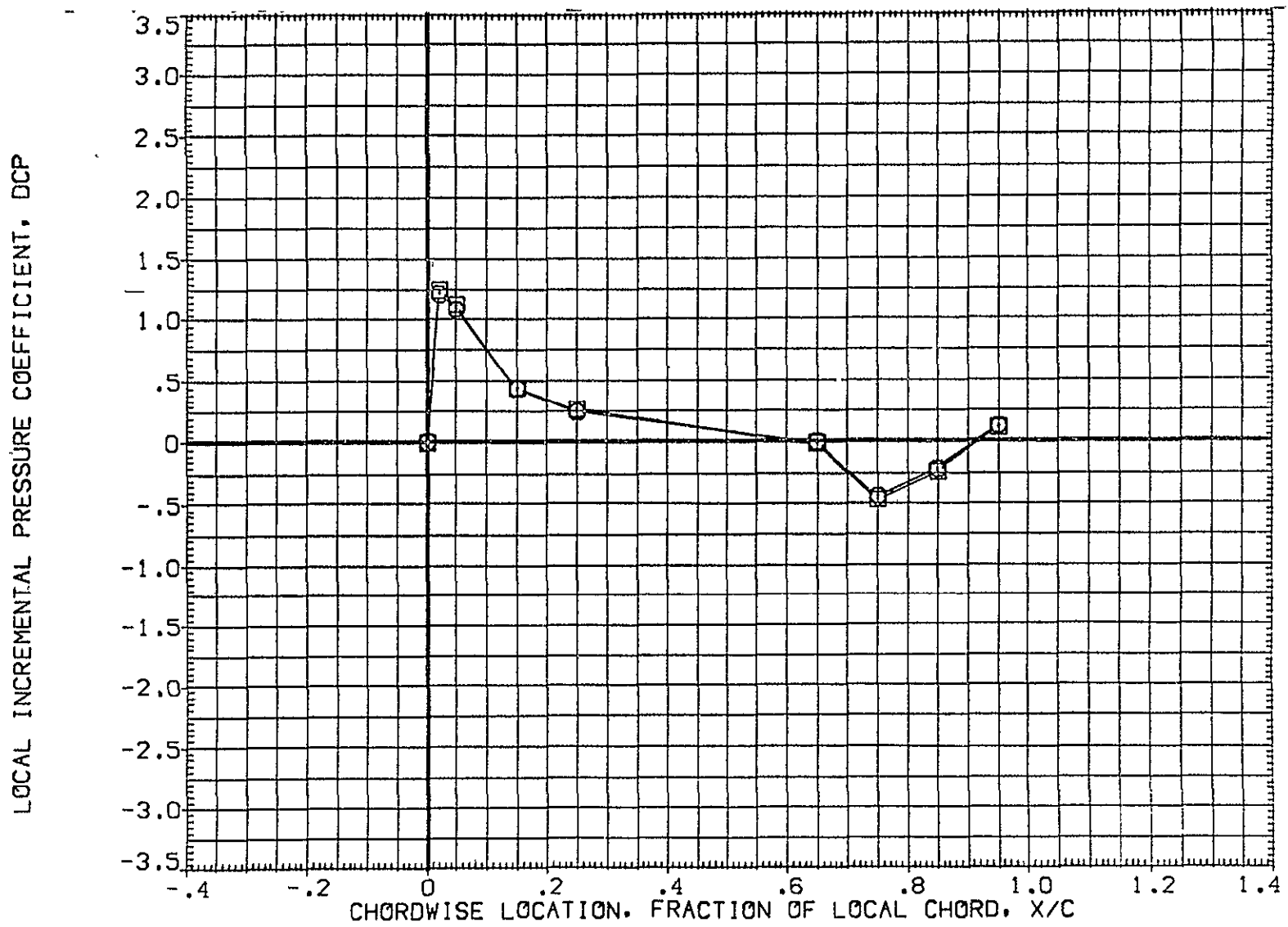
FIG 30 EFFECT OF FORWARD ATTACH POINT WEDGE, 8 DEGREE ELEVON DEFLECTION
