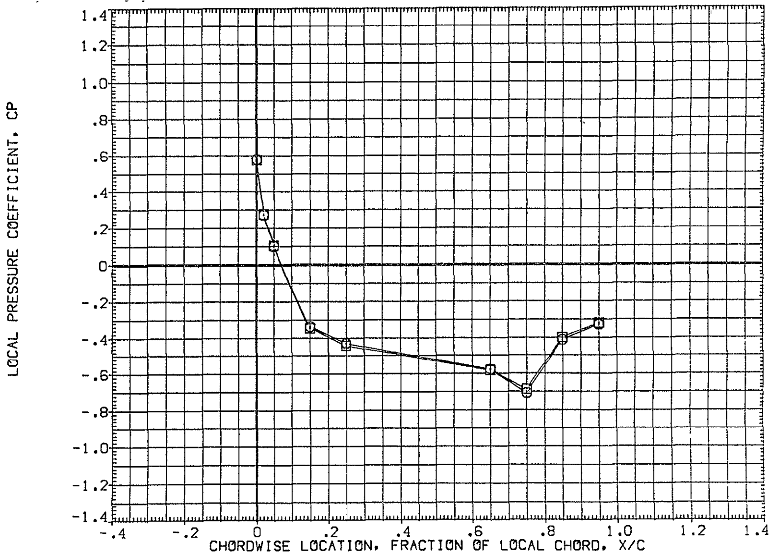
FIG 30 EFFECT OF FOREWARD ATTACH POINT WEDGE, 8 DEGREE ELEVON DEFLECTION
