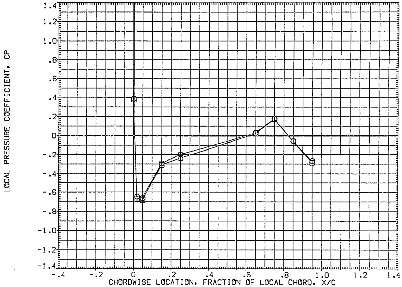
FIG 30 EFFECT OF FORWARD ATTACH POINT WEDGE, 8 DEGREE ELEVON DEFLECTION MACH = 1.240 ALPHA = -4.000 2Y/B = .771 PAGE 1300
