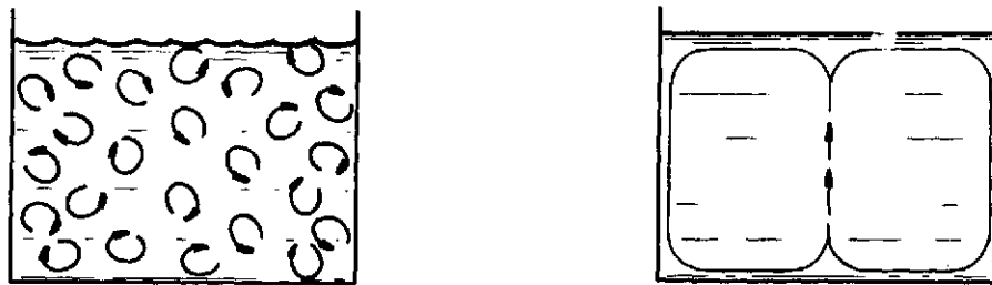
(a) Gravity driven in 1-g_0 (Turbulent) (b) Gravity driven in 10^{-6}g_0 (Laminar)
