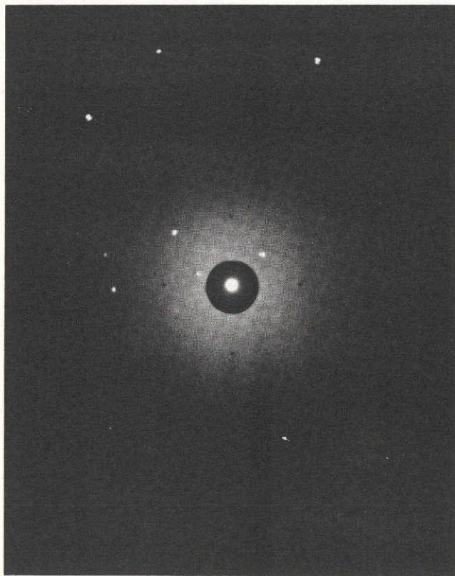
Figure 12. Comparison of Laue X-ray Patterns of Growth Regions with that of Seed for FF-98-3A (Locations 5, 10 and 16 in Figure 11B).
