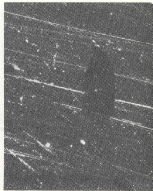
(c) Saturation coverage of chlorine; width of wear scar, 0.10 millimeter; maximum coefficient of friction, 1.0.
