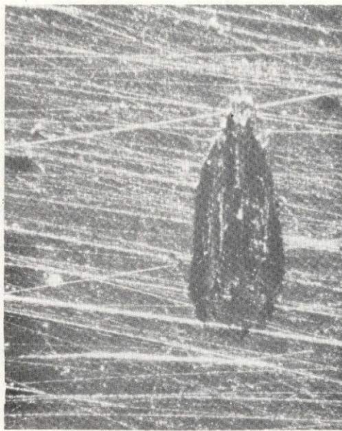
(b) Intermediate coverage of chlorine; width of wear scar, 0.13 millimeter; maximum coefficient of friction, 1.8.
