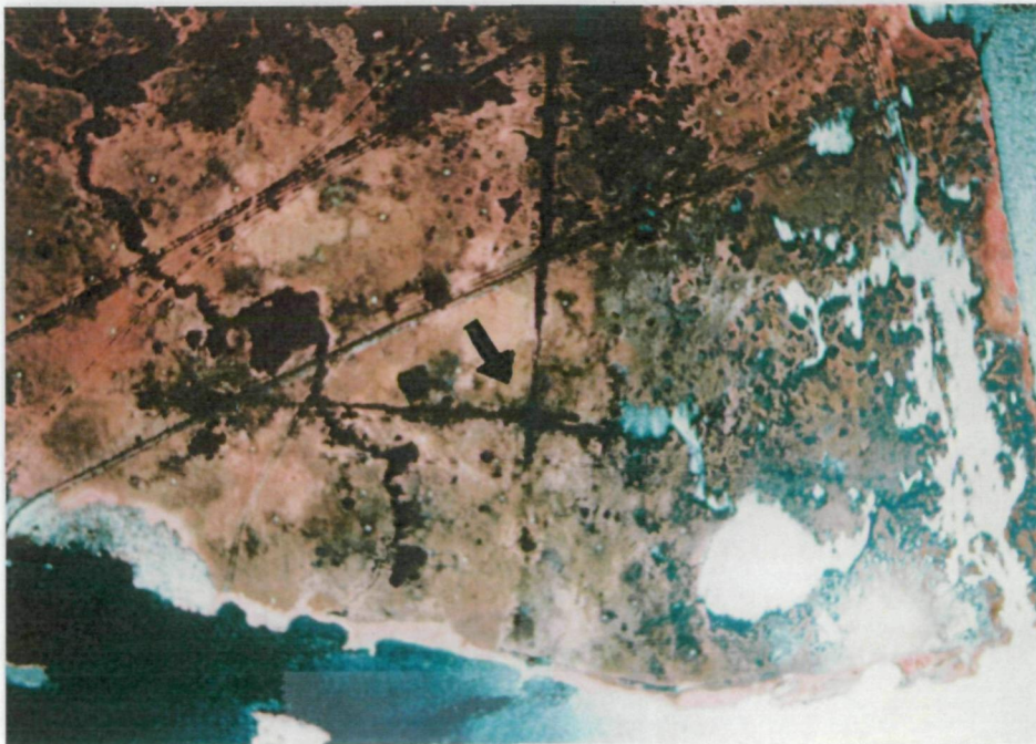
Figure 4 Continued use increases compaction and tracks become elongated water bodies
