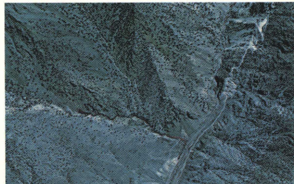
PLATE VIId — Conventional Color Infrared photograph of the same area as Plate VIIc. Fixed exposure ratio between the dye layers prevents detection of rock types and fault contacts.
