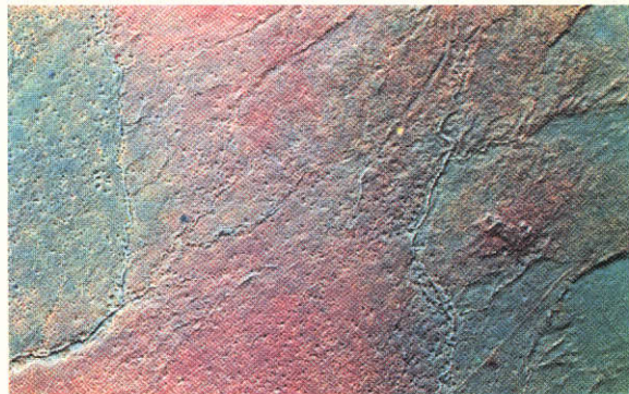
PLATE VIIb — An isoluminous rendition of the same photograph shown in Plate VIIa. The removal of all brightness differences creates an image, the color variations of which represent changes in the soil spectral distributions.
