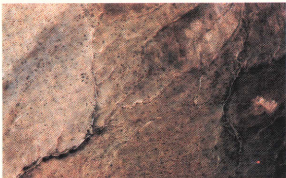
PLATE VIIa — Conventional Multispectral photograph of the Gunnison Hills area, Arizona. Varying terrain brightness causes difficulty classifying the soil-vegetation units on left and right of photo.
