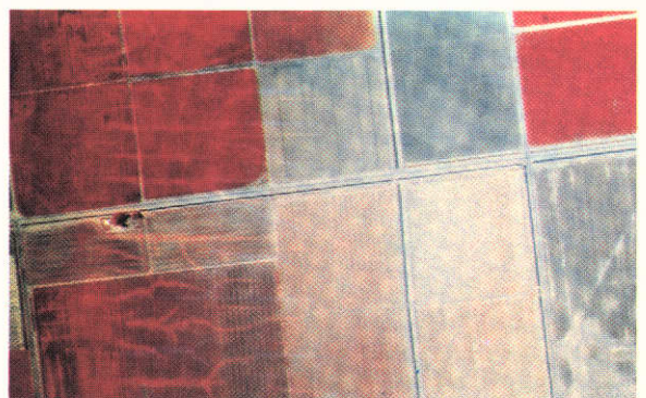
PLATE VIIIIf — Multispectral simulated Color Infrared photograph exposed over Imperial Valley, California. Bare soil, cotton and sorghum as well as alfalfa on rye grass are identified due to their unique color signatures.
