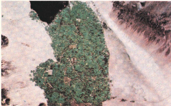
PLATE VIIIa — An additive color rendition of Apollo IX multispectral photograph #3799. The color difference between vegetation, soil and water was enhanced so that no color overlap exists between these land use categories.
