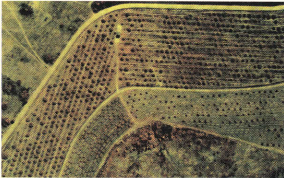
PLATE VIIIc — A conventional multispectral photograph of an avocado grove which is partially infested with root rot disease. A color difference between the healthy and diseased trees does not exist here.
