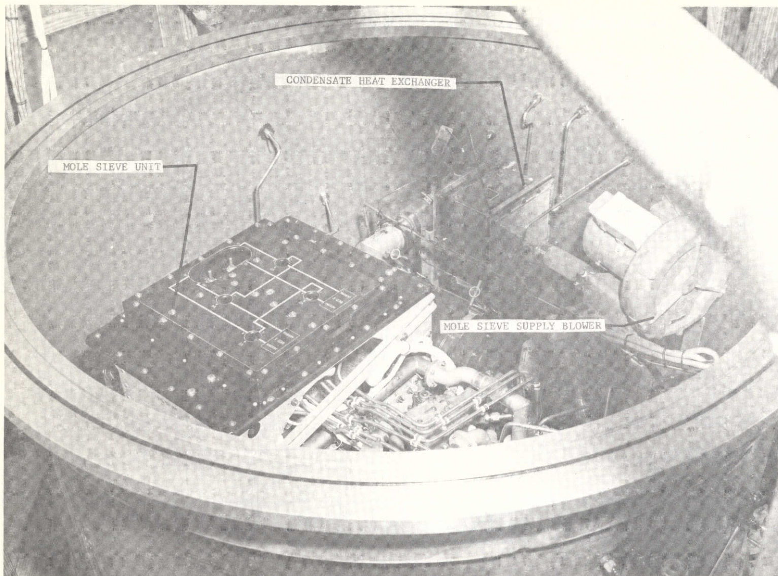
Figure 8. View of qualification unit mole-sieve test facility.
