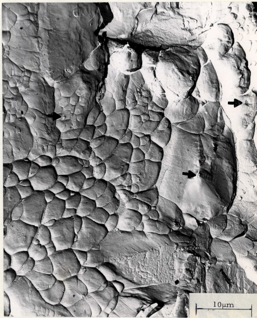
Figure 21. TEM fractograph of the air-cooled, ELI Ti-5Al-2.5Sn alloy from an LT orientated 1x1 bend K_{Ic} specimen tested at 20°K (-423°F). (Arrows point to void nucleation sites.)
