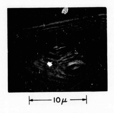
FIG. 2--SEM read out of holograms of 1.305  $\mu$  diameter particles (25 KV electron potential, 60° sample tilt).
