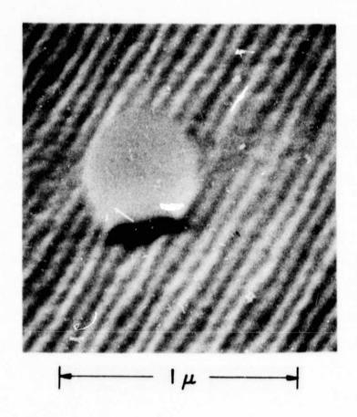
FIG. 1--SEM read out of 836 Å spaced fringes produced in PMMA by 1182 Å radiation. The round object is a 0.500 $\mu$  diameter latex sphere placed on the fringes after developmer: for magnification calibration. (25 KV electron potential, 80° sample tilt.)
