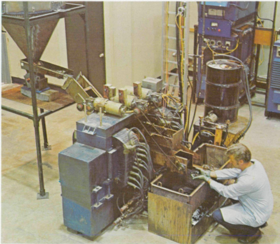
The Avco pilot plant which separates valuable nonferrous metals from scrap salvage.
