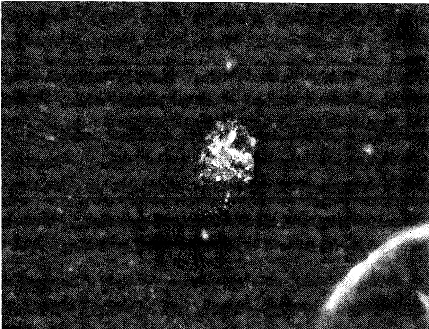
Photo #2 Silver area on bottom of Anode S/N 51. -21 300 hr. (70X)
