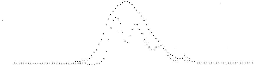
Figure 3. Digitized representation of the photographed pulses: \*= transmitted pulse; x= received pulse. Sweep duration = 100 ns.
