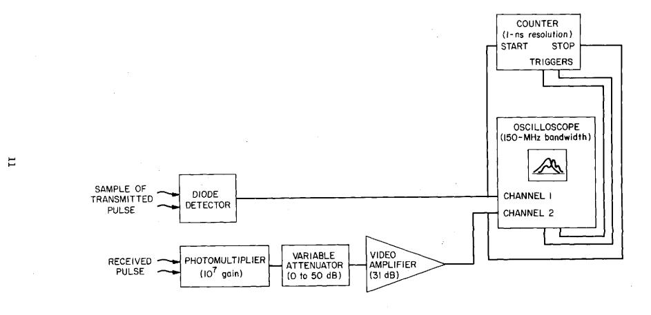
Figure 1. Block diagram for pulse detection.
