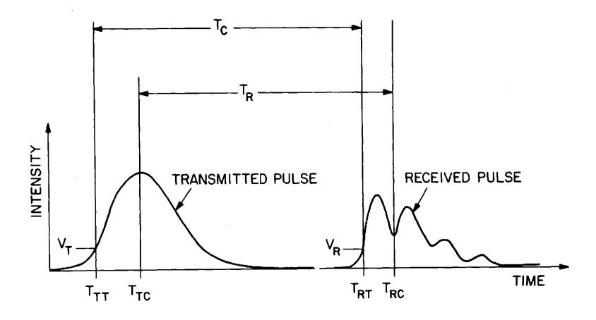
Figure 2. Diagram for the range correction  $\Delta$ , where  $T_R = T_C + \Delta$  and  $\Delta = (T_{RC} - T_{RT}) - (T_{TC} - T_{TT})$ .
