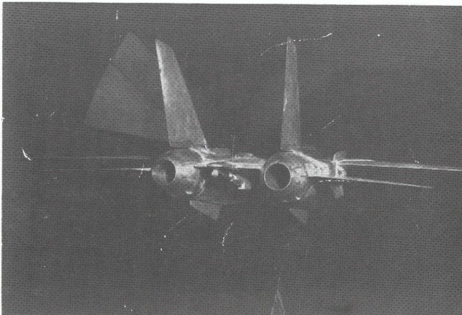
(r) Rear view of nozzle type B, cruise power setting, with interfairing 6.
